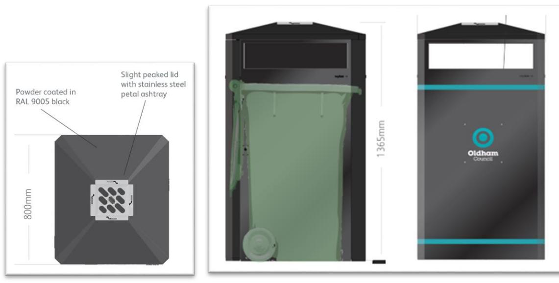
**New proposed large capacity metal bin housings containing a standard 240 litre standard wheeled refuse bin.**
